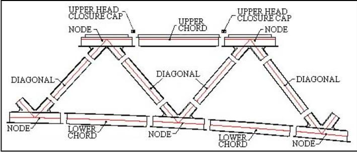
*Fig. 8.* Break-down into simple elements for shop manufacture
