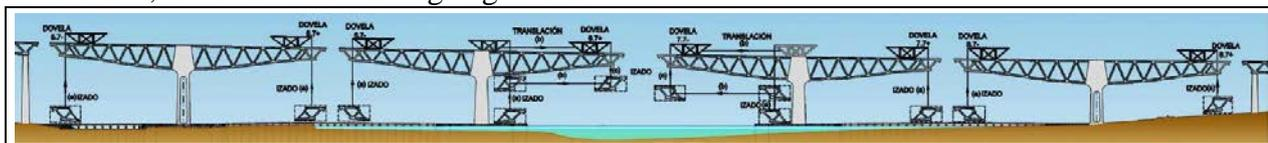
Fig. 4. Scheme of the constructive procedure by incremental equilibrated cantilevers
