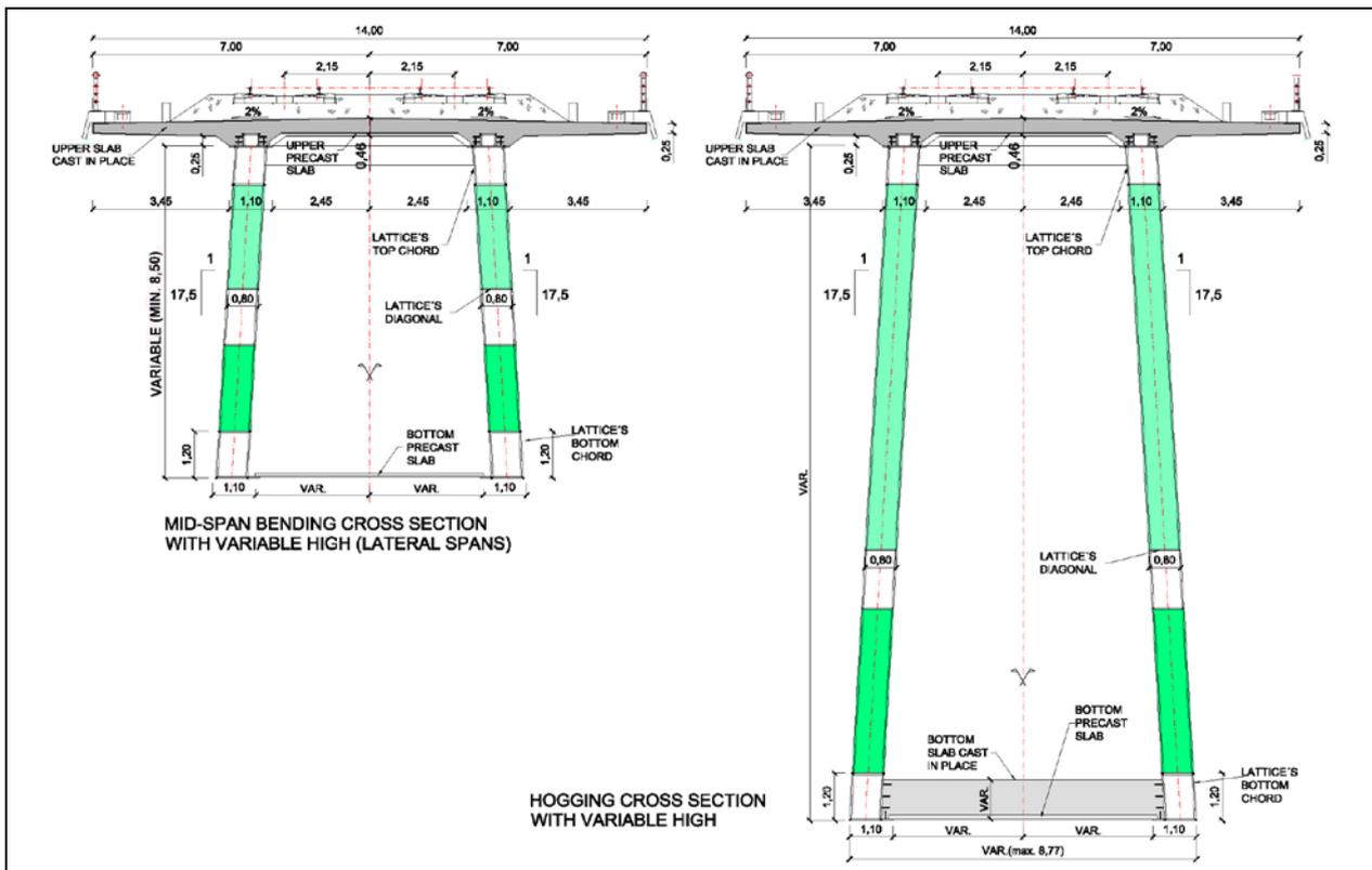
*Fig. 2.* Sagging cross sections and hogging cross section in the variable depth central zone
