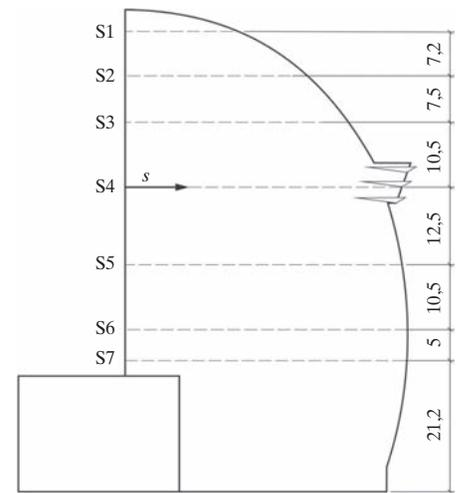
Fig. 6: Instrumented cross sections,  $s$  is the horizontal distance of each cross section S1 to S7
