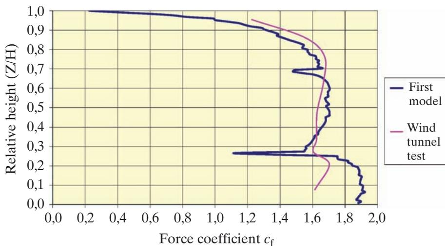
Fig. 8: Force coefficient of the building reproducing the actual geometry of the wind tunnel
