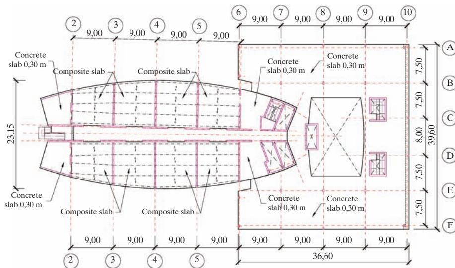
Fig. 2: Typical plan view between level 1 and level 7 of the Tower and the Atrium (Units: m)
