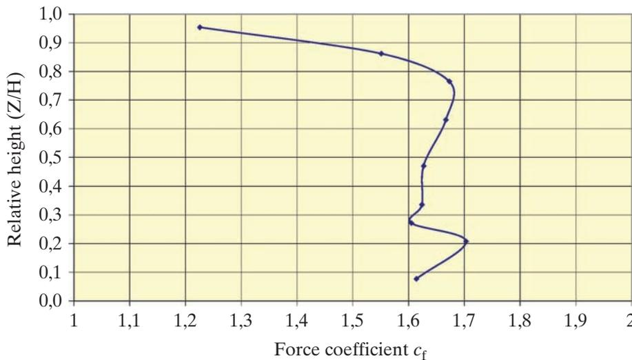
Fig. 4: Force coefficient with transverse wind
