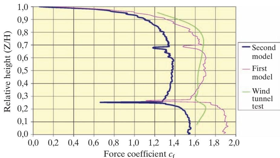
Fig. 10: Force coefficient of the building in open field without any restriction for the wind
