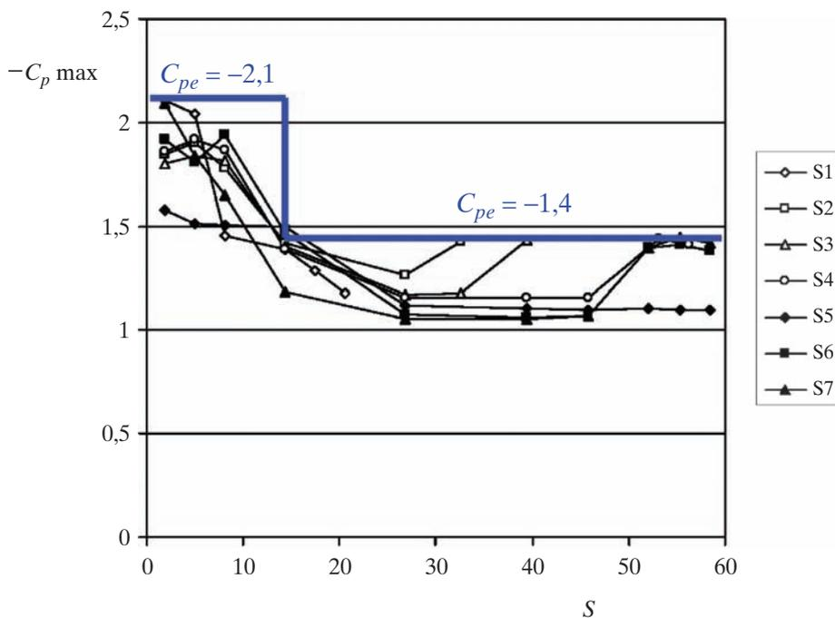
Fig. 5: Maximum suction pressure in the facade, Horizontal axis:  $s$  is the distance according to Fig. 6. Vertical axis:  $-C_p \max$  is maximum (negative) external pressure coefficient (suction).
