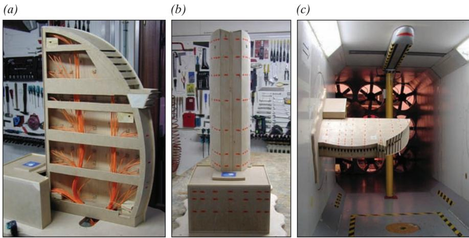
Fig. 3: (a, b and c) Views of the model in the interior of the wind tunnel
