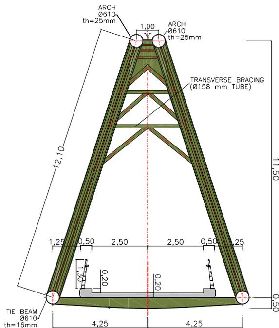
Fig. 18 N-II Footbridge (80 m). Cross section
