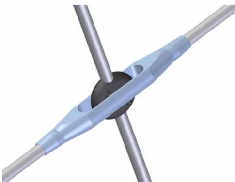
*Fig.4 Deba Bridge. Hanger crossing device (2006)*
