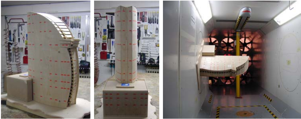
Figures 4a, 4b & 4c: Views of the model in the interior of the wind tunnel.
